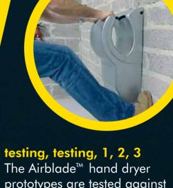
The Airblade<sup>™</sup> hand dryer prototypes are tested against the specification for hygiene, efficiency, speed and noise levels. Fresh chickens are used to contaminate volunteers' hands prior to washing, drying, then microbiological skin testing.
