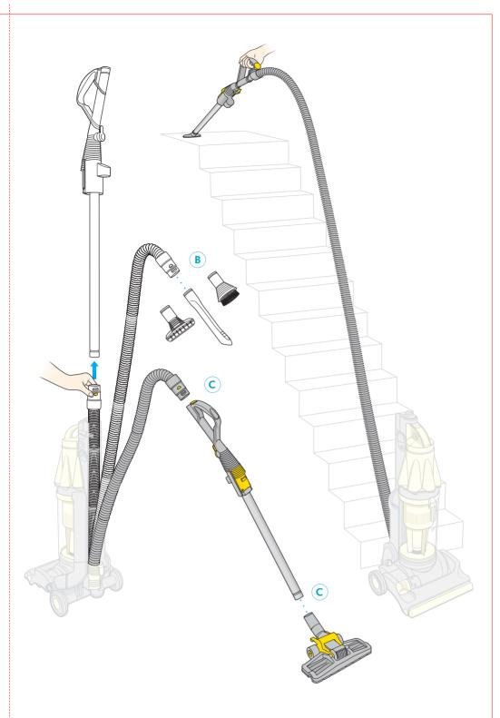
Press wand release button and remove wand.
