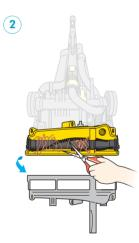
Tilt machine forward and slide out U-bend airway inspection **B**. Check inside for blockages.
