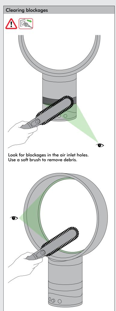
Look for blockages in the small aperture inside the loop amplifier. Use a soft brush to remove debris.
