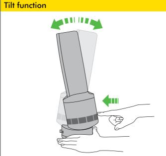
Adjust base forward or backward for required airflow angle.
