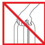
Do not carry by the air loop amplifier. The air loop amplifier is not a handle.
